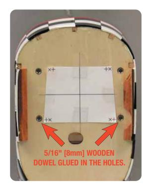
4. The bolts included with the DLE engines are too short to pass through the firewall and spacers. 10-32x 2" [50mm] Socket head cap screws, #10 lock washers and #10 fender washers will be required to mount the DLE engine. The bolts included with the O.S. 2" [50mm] standoffs are also too short. 5x40mm Socket head cap screws are required.
